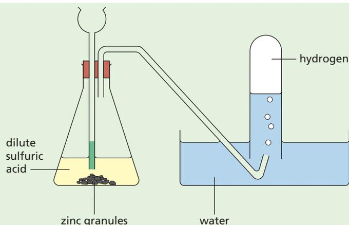
**Figure 12.8** The laboratory preparation of hydrogen gas.
