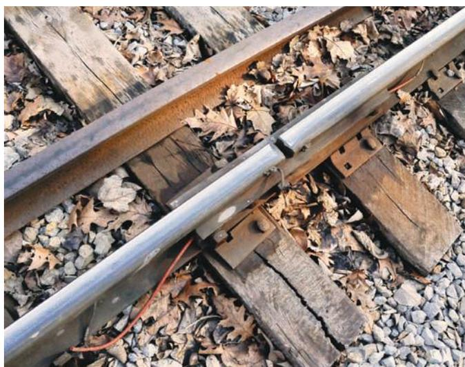
**Figure 1.2** Without expansion gaps between the rails, the track would buckle in hot weather.
