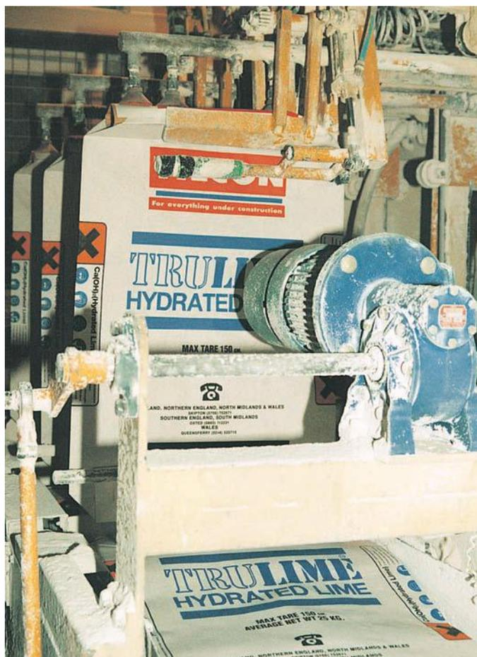
Figure 13.9 Large-scale production of calcium hydroxide.
