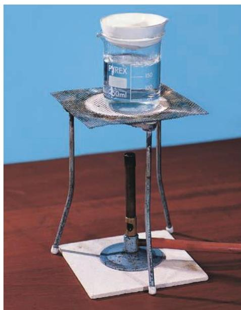
**Figure 2.16** Apparatus used to slowly evaporate a solvent.
