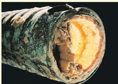
**b** The thick deposits of limescale can be seen in this hot water pipe.
