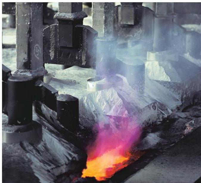
**c** Aluminium is produced by electrolysis.
