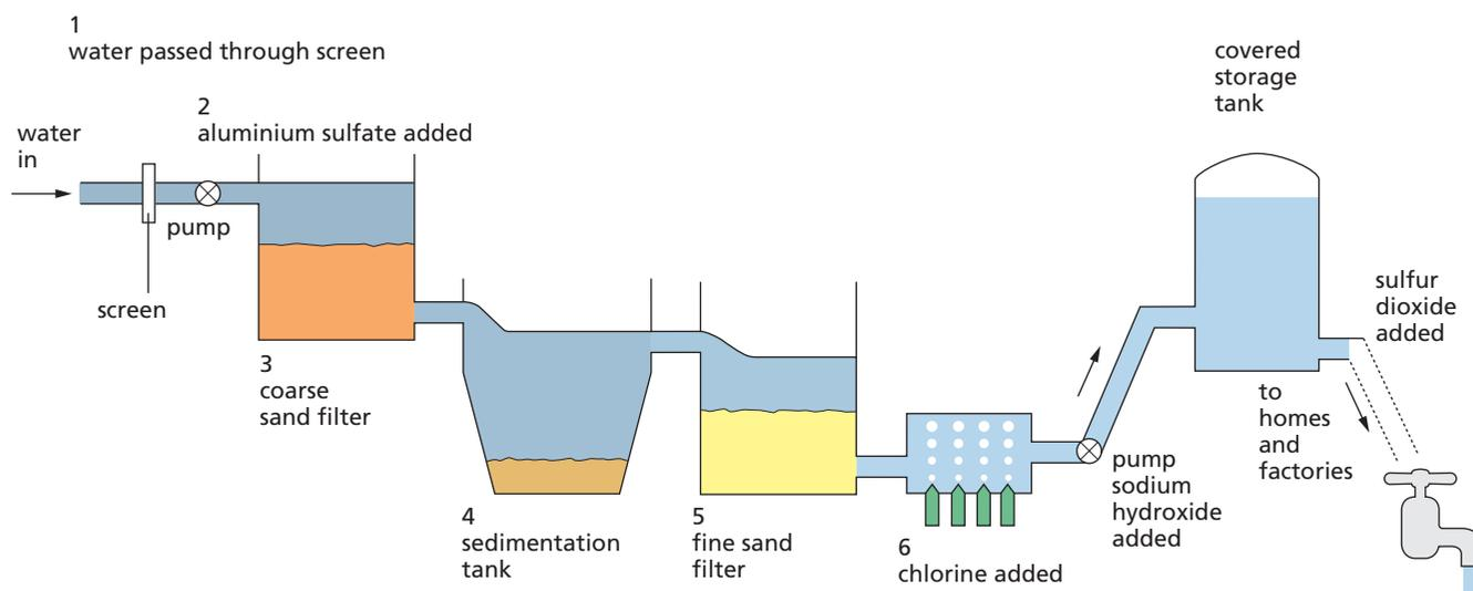
Figure 11.39 The processes involved in water treatment.
