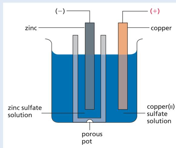
It is capable of generating about 1.1 volts and was used to operate small electrical items such as doorbells.
