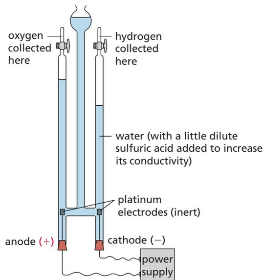
**Figure 5.11** A Hofmann voltameter used to electrolyse water.
