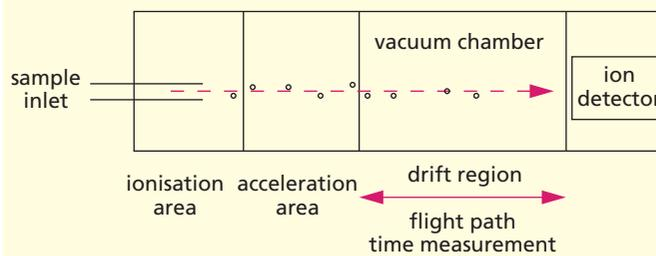
**Figure 3.6** A diagram of a mass spectrometer.
