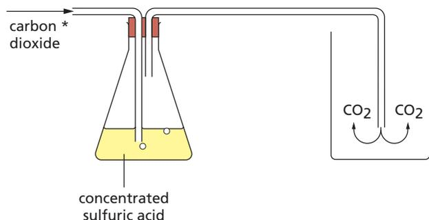
Figure 13.16 Preparation and collection of carbon dioxide gas.
