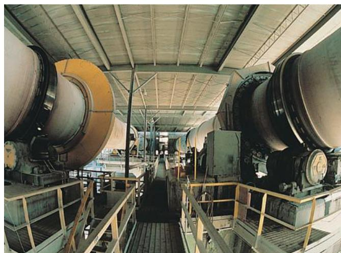
Figure 13.5 A modern rotary kiln.
