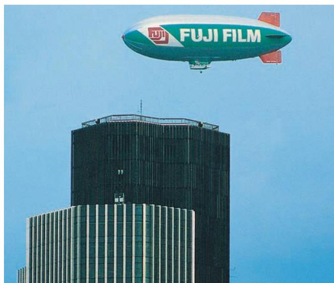
**Figure 11.12** Helium is used to fill this airship as it has a low density and is unreactive.
