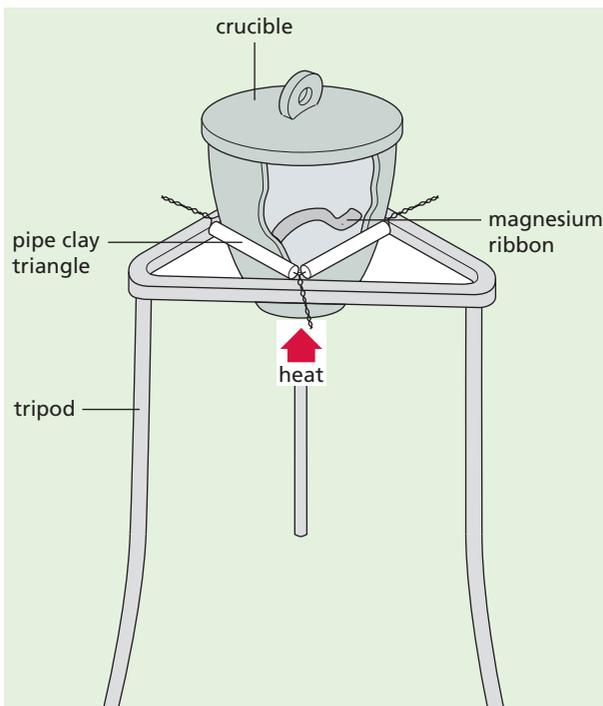
**Figure 4.5** Apparatus used to determine magnesium oxide's formula.
