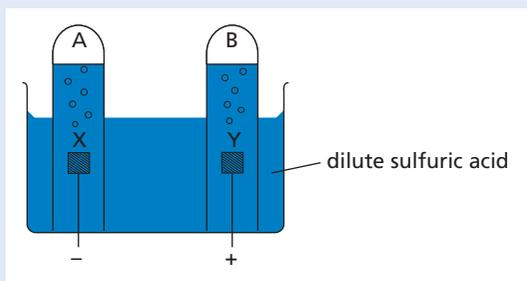
This is a diagram of an experiment in which electricity was passed through a mixture of distilled water containing a little dilute sulfuric acid.
