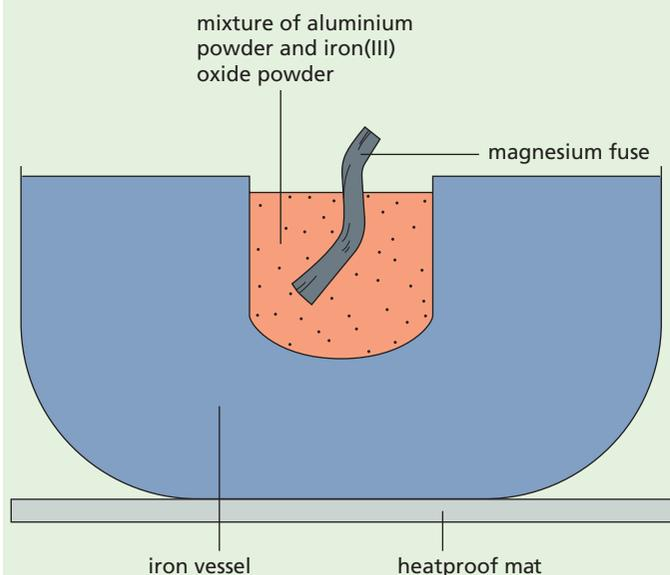
Figure 10.6 Themit reaction mixture apparatus.
