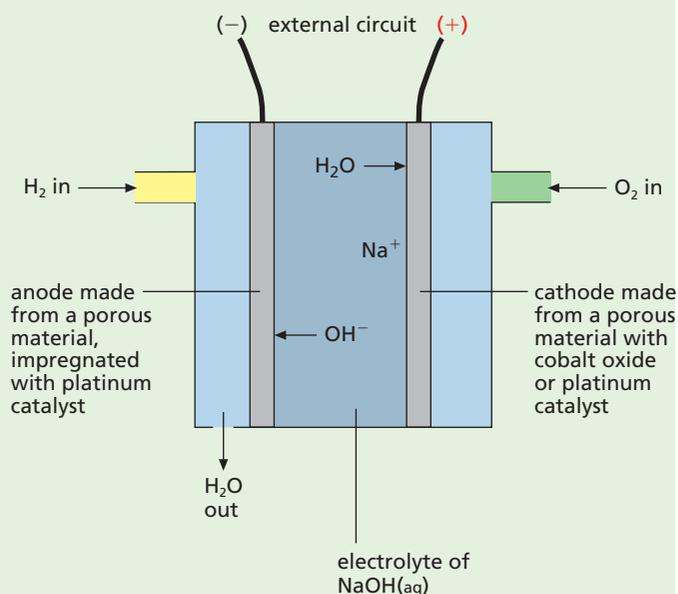
**Figure 6.25** A diagrammatic view of a fuel cell.
