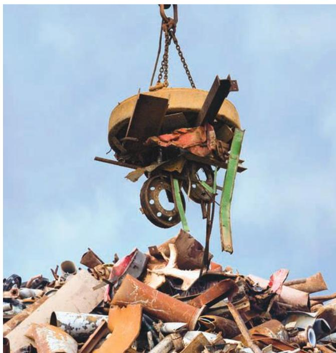
Figure 2.24 Magnetic separation of iron-containing materials.
