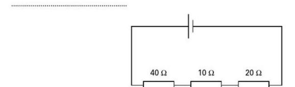
c Calculate the combined resistance of the three resistors in the circuit in part b above.
