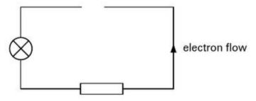
arrow shows the direction in which the electrons move in the circuit.
