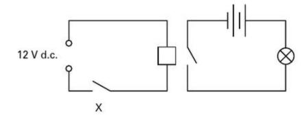
c Copy the circuit symbol for the relay into the space below. Label the parts of it that represent the coil and the switch.
