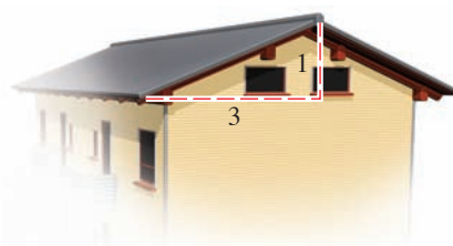
Pitch of a roof Slope = \frac{1}{3}
